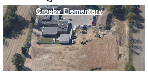
All Schools: Mass excavation and grading have been completed at all sites, and the building pads, parking lots, and roads have been cement stabilized. Installation of utility piping for storm water drainage, sanitary waste, and water distribution continues.
